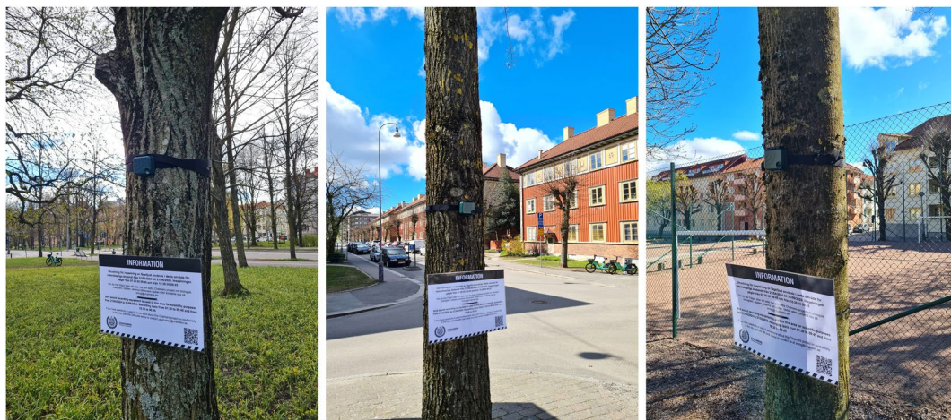
Fig. 3 AudioMoth recorders housed in IPX7 waterproof cases and strapped to tree trunks in different study sites in Gothenburg, Sweden.
