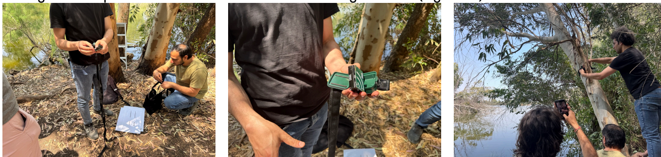
Figure 4. Demonstration of configuration and placement of sensors during site visit
