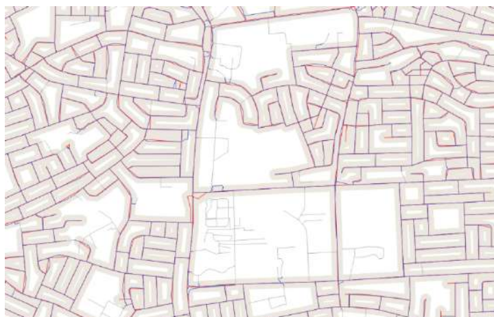
Figure 9. For the sensitivity analysis, we selected the automated model (blue lines) that only falls within a 25 m buffer from the hybrid model (red lines), creating a buffered model. (Grey lines are the ignored lines from the automated model)
