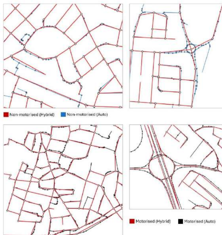
Figure 12. Difference in representation (segments & nodes) between the two models, the upper images represent the non-motorised, and the lower images represent the motorised
